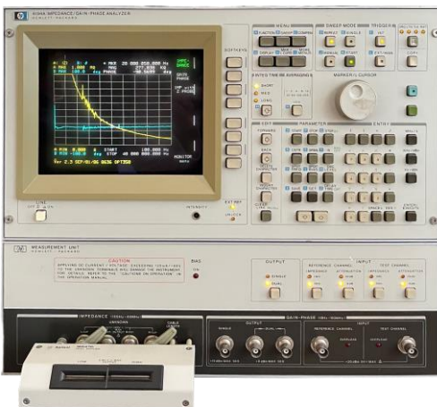
LRC bridge (HP 4194A)
