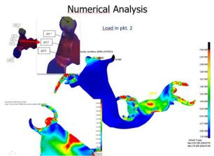
The boundary conditions and loading of the denture structure has been modelled in this programme in order to determine the stresses and strain. The results of calculation are presented in graphical form.
