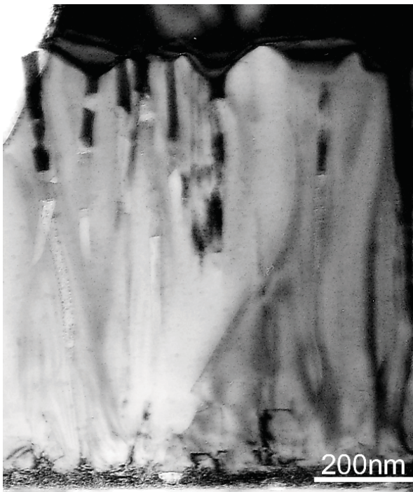
Fig. 2.8. Typical structure of GaN layers after annealing in Zn vapor at temperature of 1200°C.
